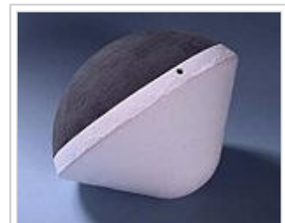
DS/2 aeroshell, a classic 45° sphere-cone with spherical section afterbody enabling aerodynamic stability from atmospheric entry to surface impact
