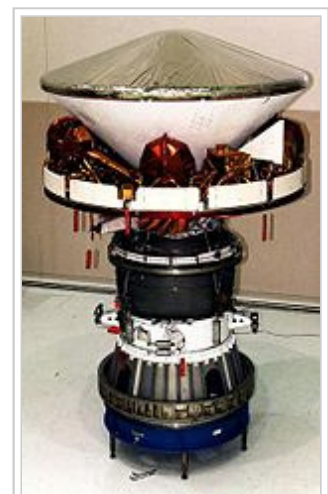
Mars Pathfinder during final assembly showing the aeroshell, cruise ring and solid rocket motor
