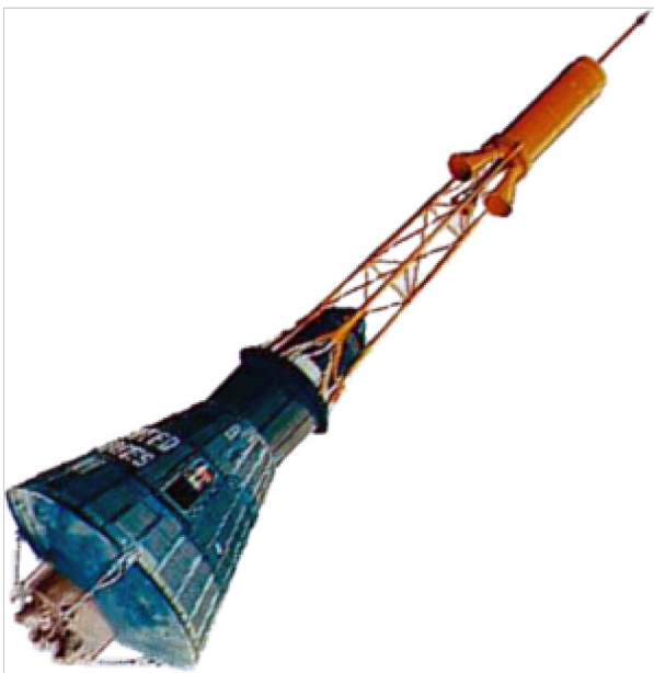
The Mercury Capsule design (shown with escape tower) originally used a radiatively cooled TPS but was later converted to an ablative TPS
