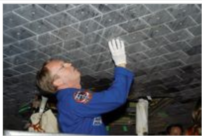
Astronaut Andrew S. W. Thomas takes a close look at TPS tiles underneath Space Shuttle Atlantis.
